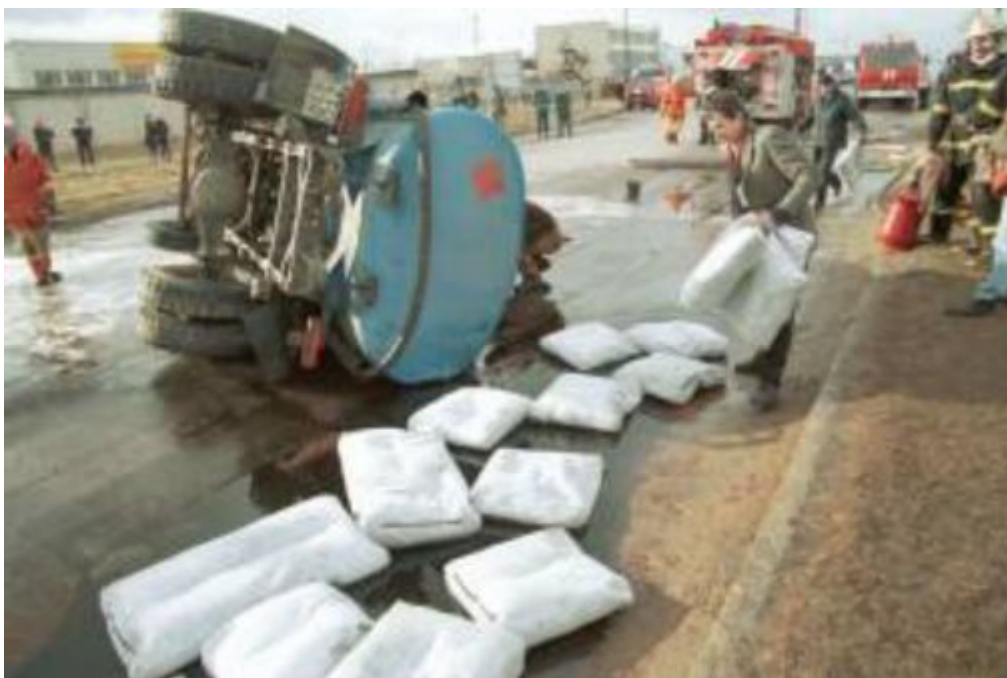
Liquidation of emergency POL spills using HRCM in Shaulyaj, Lithuania. Fire engines are equipped with special HRCM-filled pads.
