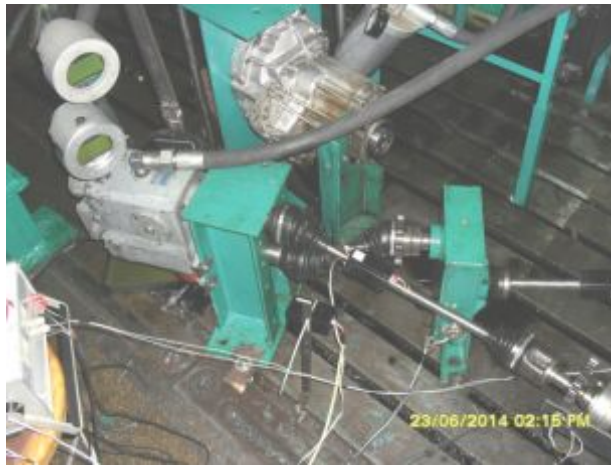
Fig. 2 – Appearance of stand №1 for studying HST
