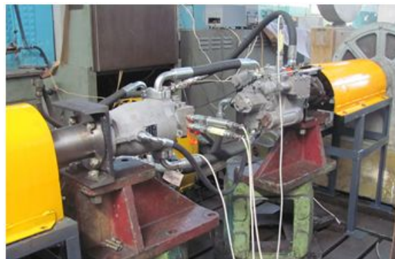
Fig. 4 – Appearance of stand №2 for studying HST
