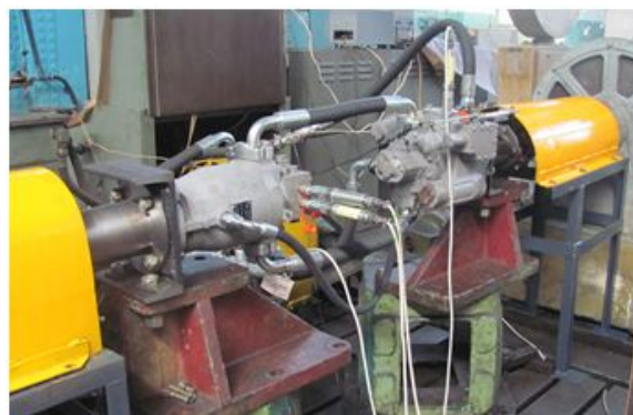
Fig. 4 – Appearance of stand №2 for studying HST
