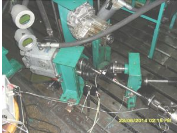
Fig. 2 – Appearance of stand №1 for studying HST
