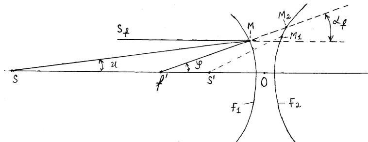
$S_f$  - beam from infinitely remote object,  $f'$  - imaginary focus.
