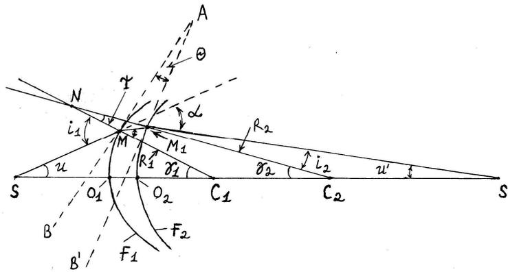
Figure 2 – Scheme of a thin lens. Convexities of surfaces  $F_1$  and  $F_2$  have the same left-left orientation.
